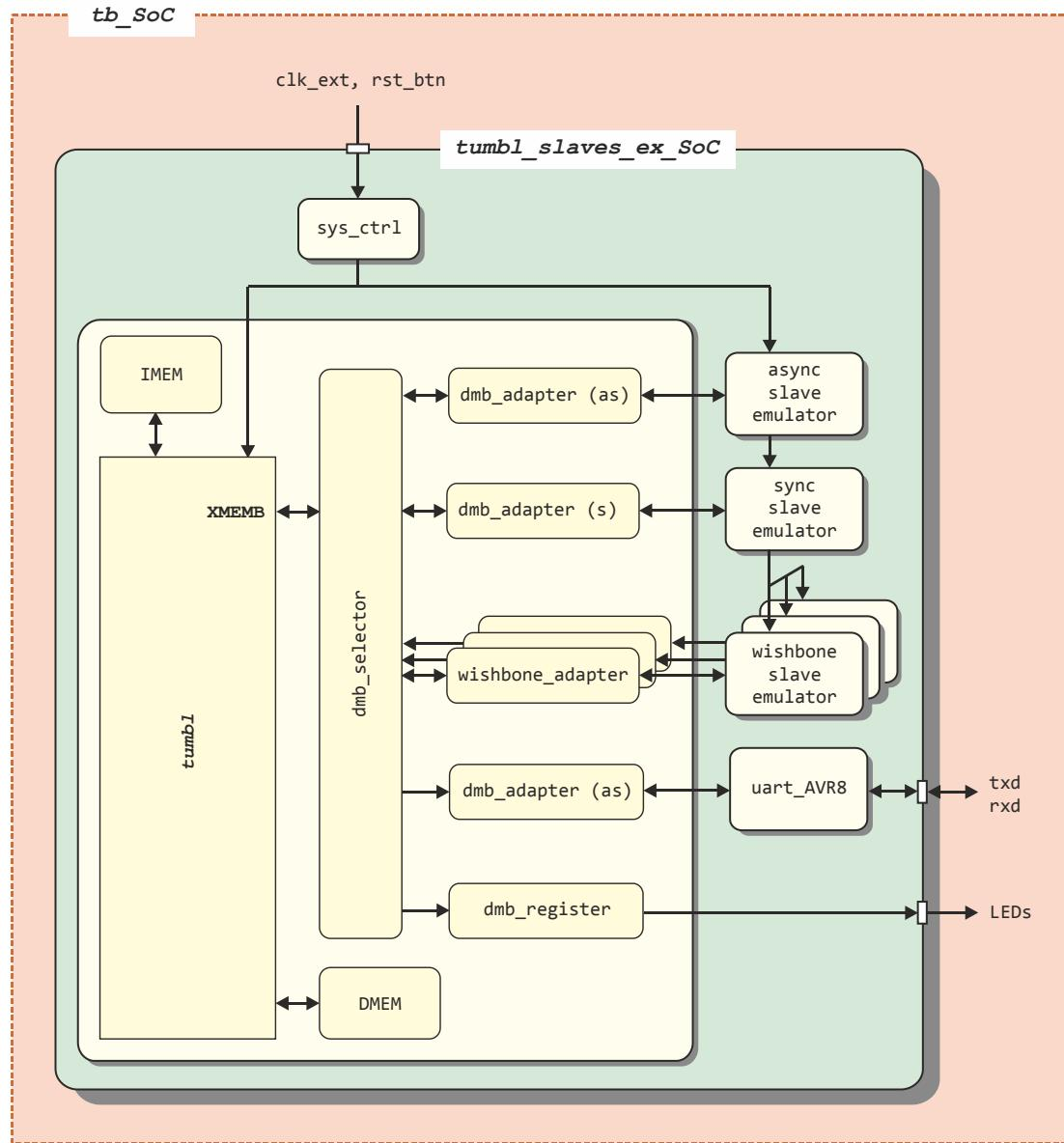
**Figure 5.4** Block diagrams of the `tumbl_slaves_ex_SoC` and its testbench.
