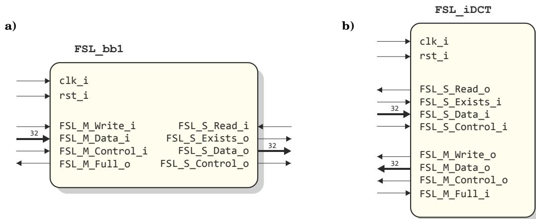
**Figure 4.1** Block diagrams of a) the `fsl_bb1`, and b) the `fsl_idct` components.
