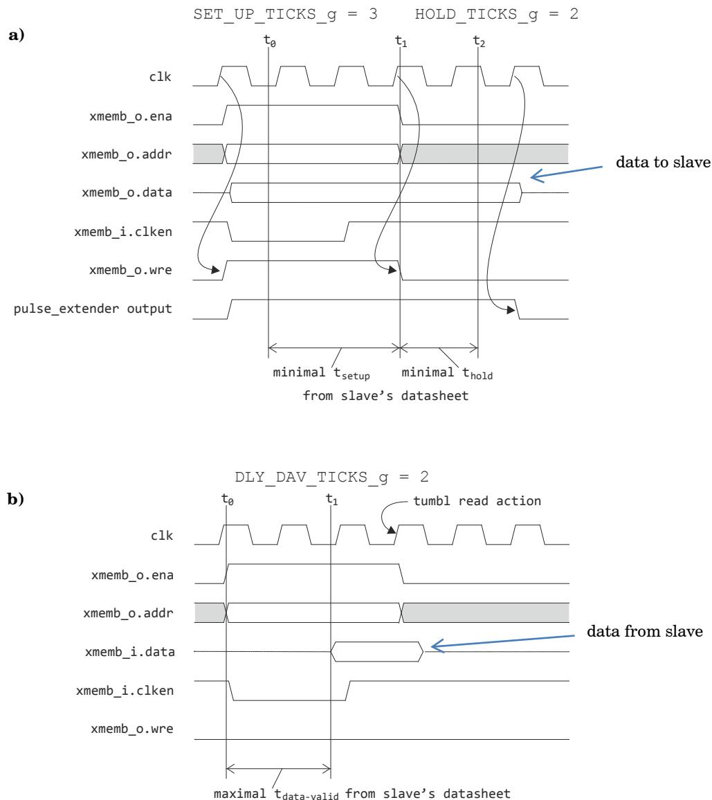
**Figure 5.3** Examples of specific timing needed for a) writing to, and b) for reading an off-chip component.
