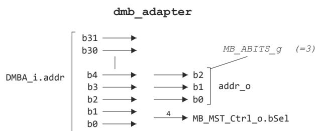
**Figure 5.2** Address mapping between `tumb1` and memory mapped slaves in the `dmb_` and `wb_` adapters.
