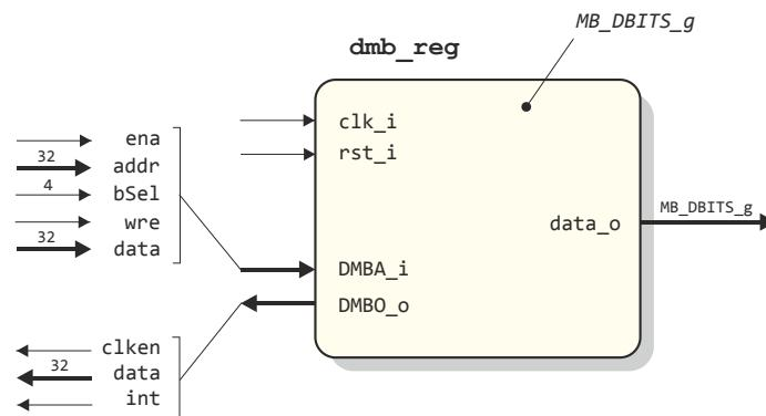
**Figure 5.7** Block diagrams the `dmb_reg` component.
