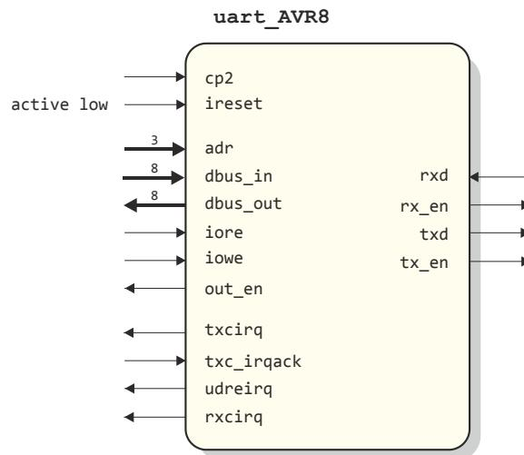
**Figure A.1** Block diagram of the `uart_AVR8`.
