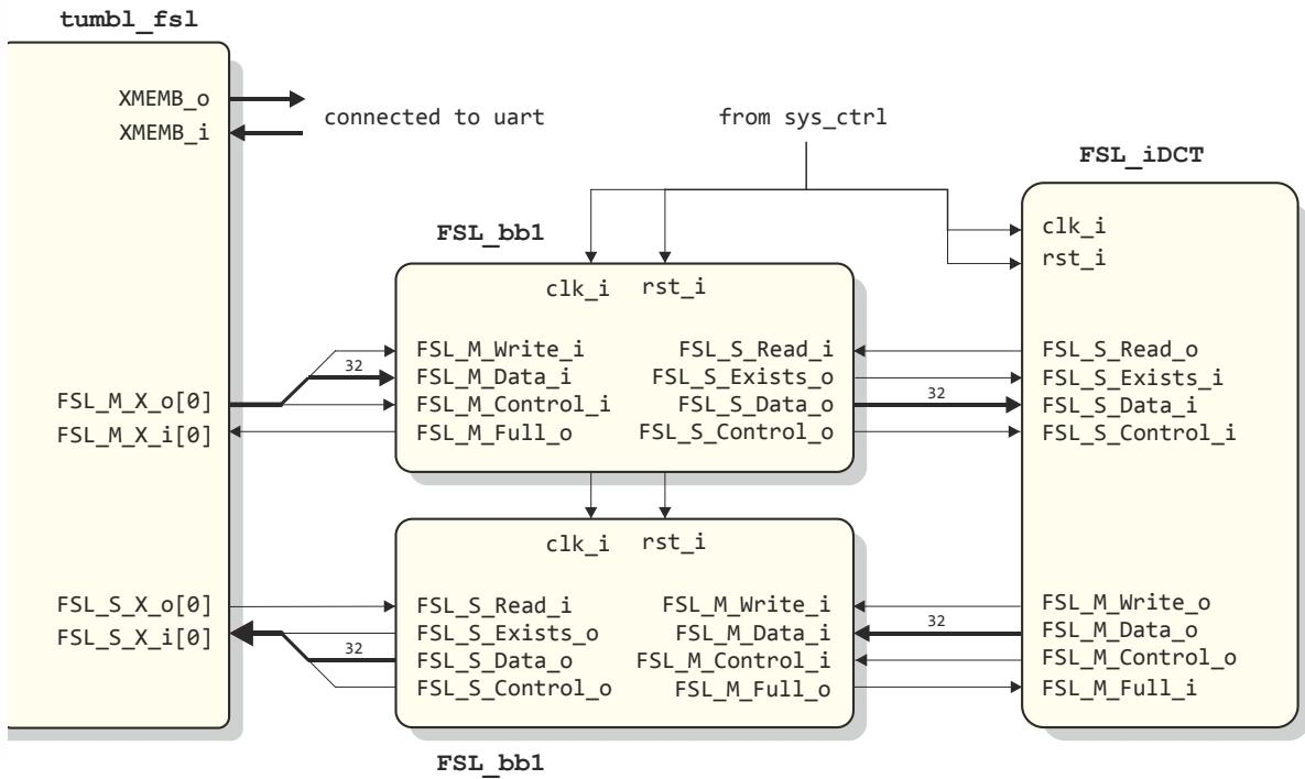
**Figure 4.2** Setup of the `tumb1_fsl` with the `idct` module and two bus interfaces.
