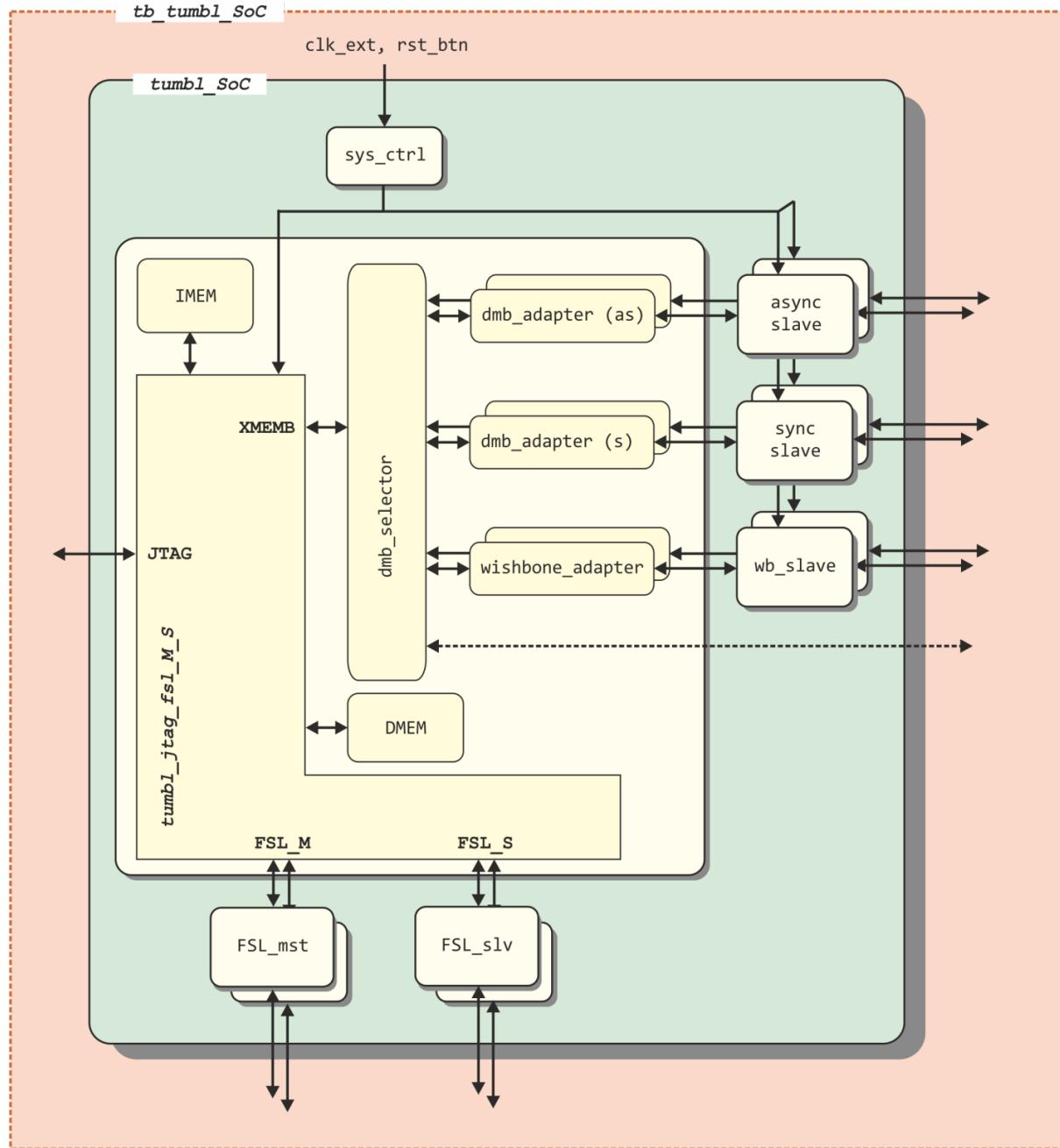
**Figure 1.1** Example scheme of a SoC with an MB-Lite+ with JTAG i/o and connections to synchronous and asynchronous slave interfaces, wishbone slaves, as well as FSL\_master- and FSL\_slave-interfaces.
