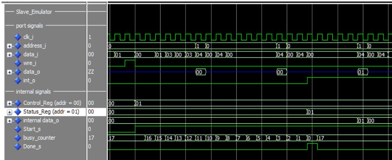
**Figure 5.6** Showing the emulation of a “busy” slave for a `DLY_BUSY TICK g` value of 17.
