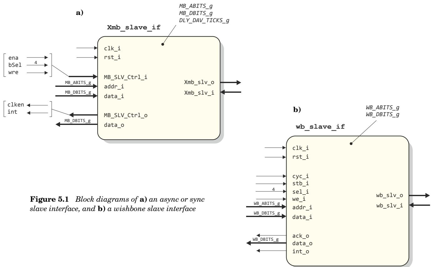
**Figure 5.1** Block diagrams of a) an async or sync slave interface, and b) a wishbone slave interface
