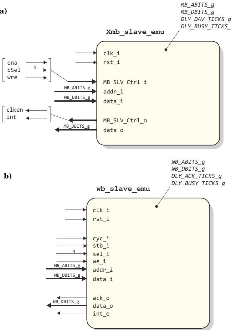
**Figure 5.5** Block diagrams of a) the `Xmb_slave_emu` where `X` can be `a` or `s`, and b) the `wb_slave_emu` components.
